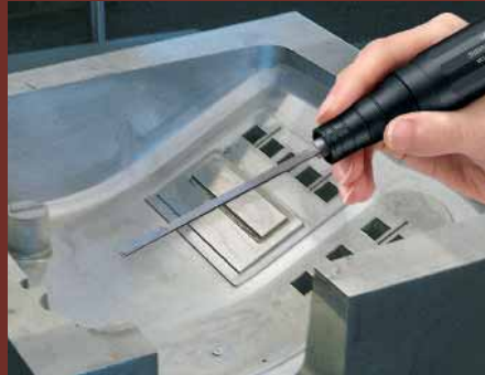
Exclusive Tools for Ultrasonic Polisher "Sheenus ZERO"
